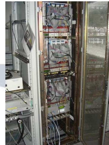
↘ CERN transverse and longitudinal feedbacks: they employ VME digital processing boards equipped with ADC, DAC, FIFOs and PLDs
