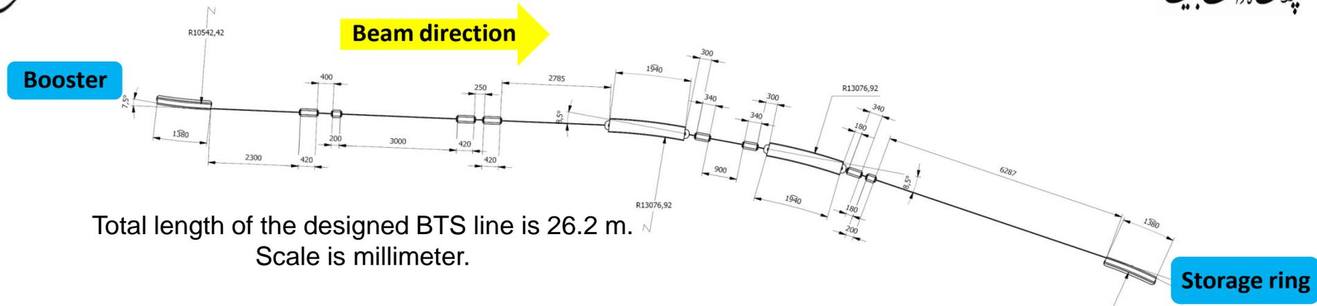
Total length of the designed BTS line is 26.2 m.
