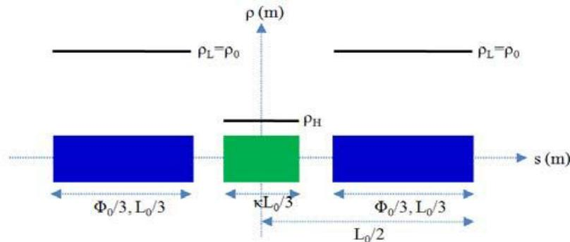
$L_0$  and  $h_0$  are the length and the curvature of the low field dipoles (B1 or B2 or B3) in the bare lattice respectively. The  $\kappa$  factor represents length ratio of high field (HF) and low field (LF) dipoles ( $L_H = \kappa L_0 / 3 = \kappa L_{LF}$ ) and indicates how far the high field section can be extended.  $N$  is the number of super period,  $n$  is the number of high field inserted dipole.
