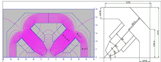
Figure 5: Field lines and dimensions of ILSF quadrupole.
