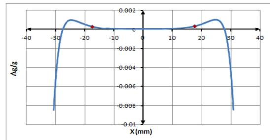
Figure 6: Field tolerance of ILSF quadrupole magnet boundaries of the good field region ( $\pm 18\text{mm}$ ) are shown in red.
