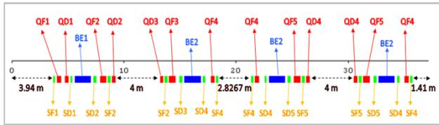
Figure 1: Arrangement of the magnets in a half-superperiod of ILSF storage ring.
