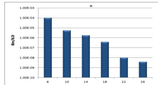
Figure 7: Absolute normalized multipoles' error at radius of 20mm.
