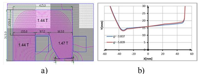
Figure 2: a) General dimensions for both BE.1 and BE.2. b) BE.1 and BE.2 pole profiles.
