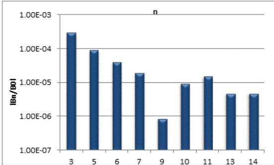
Figure 4: Absolut normalized multipoles' error at radius of 15 mm.
