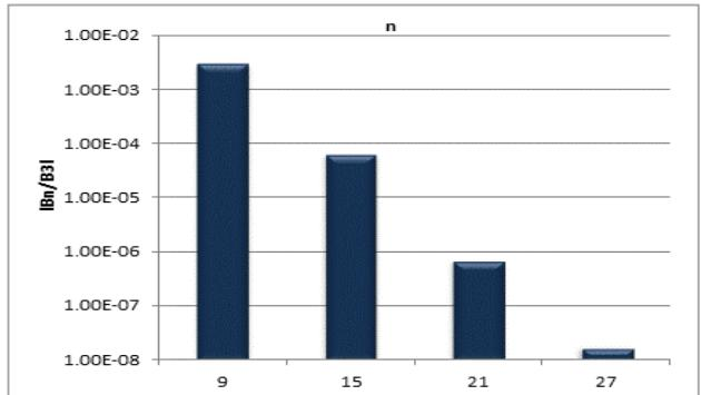
Figure 10: Absolute normalized multipoles' error at radius of 20mm.
