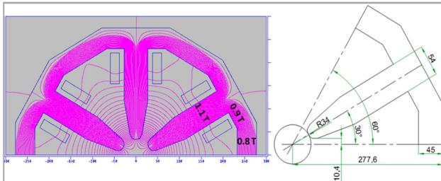
Figure 8: Field lines and dimensions of ILSF sextupole.
