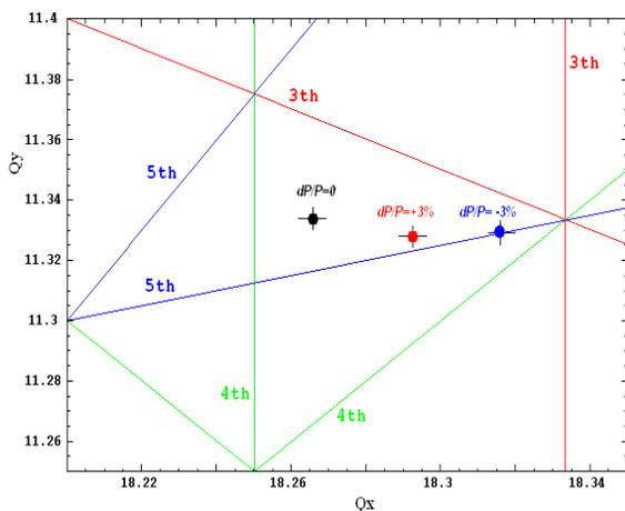
Figure 6: Working point of ILSF lattice with SCW-31 for on/off momentum.
