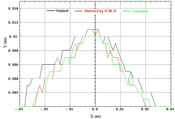
Figure 3: Dynamic aperture at the center of long straight section of ILSF ring with/without SCW-31.
