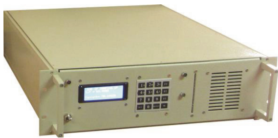
Figure 3: Fabricated 1.2 kW prototype power supply at ILSF using low resolution.
