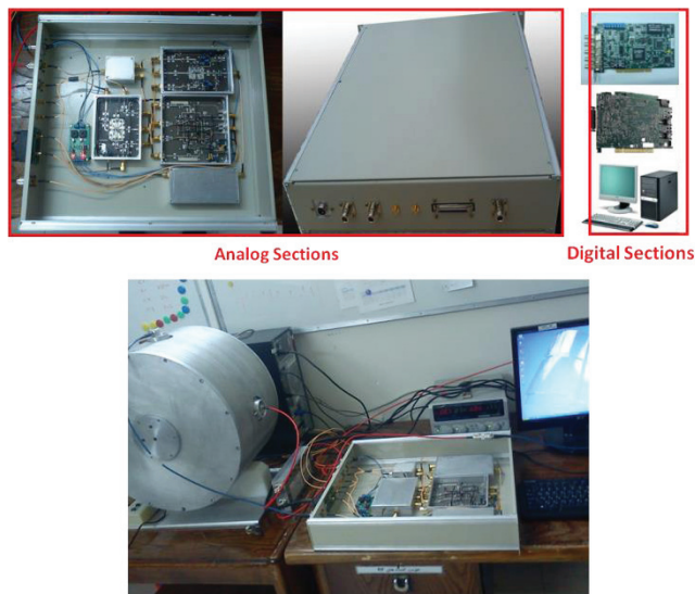
Figure 5: Analogue and digital sections of semi digital LLRF system prototype (up), system under test using an aluminium pillbox cavity (down).
