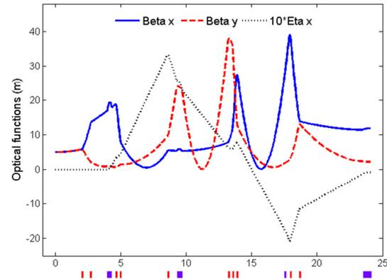
Figure 4. The optical functions along the LTB line with the initial Twiss functions of  $\beta_x=\beta_y=5$  m and  $\alpha_x=\alpha_y=0$ .
