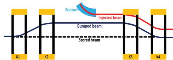
Figure 1: Schematic drawing of the injection equipment into the ILSF ring.
