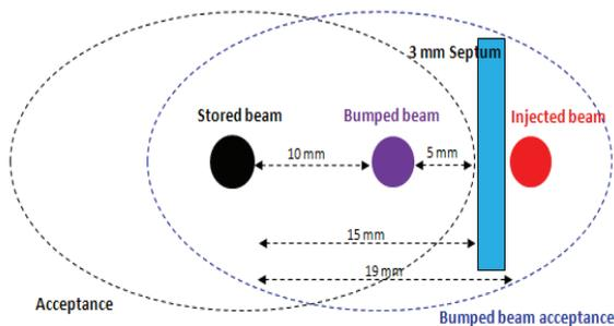
Figure 3: The reserved space for the stored, bumped and injected beams.
