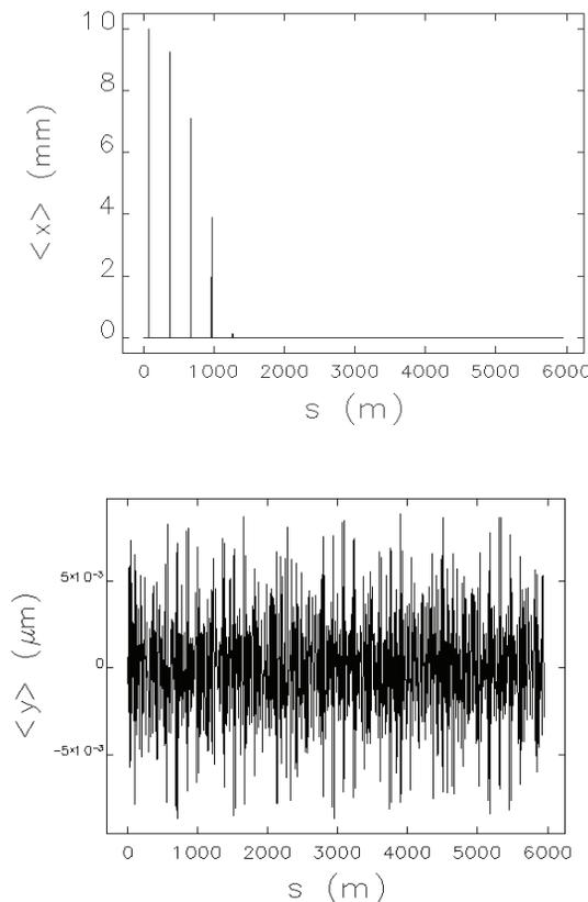
Figure 4: (top) Horizontal, (bottom) vertical trajectory of the electron beam centroid during 20 turns passing through the kicker magnets. No errors have been assumed in operation of the kickers.
