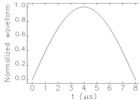
Figure 2: Normalized half waveform of the kicker magnets.
