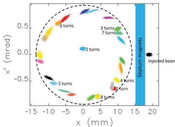
Figure 6: Phase space coordinate of the matched injected beam during 25 turns passing through the ring. Color in phase space graph indicates to the number of turns.
