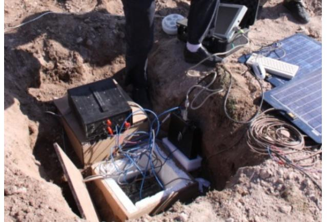
Figure 4: Installation of seismometer.
