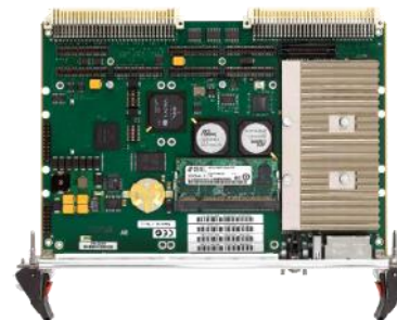
VME Card: Eurocard size VMEbus interface
